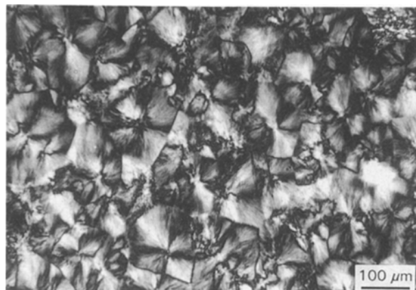
Figure 1 Spherulite morphology in the extruded polypropylene.
